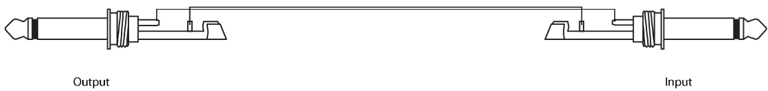
Cable to unbalanced input from unbalanced output. TS connectors.
