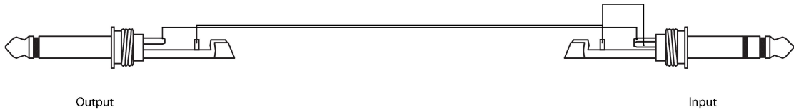
Cable to balanced input from unbalanced output. TS and TRS connectors.
